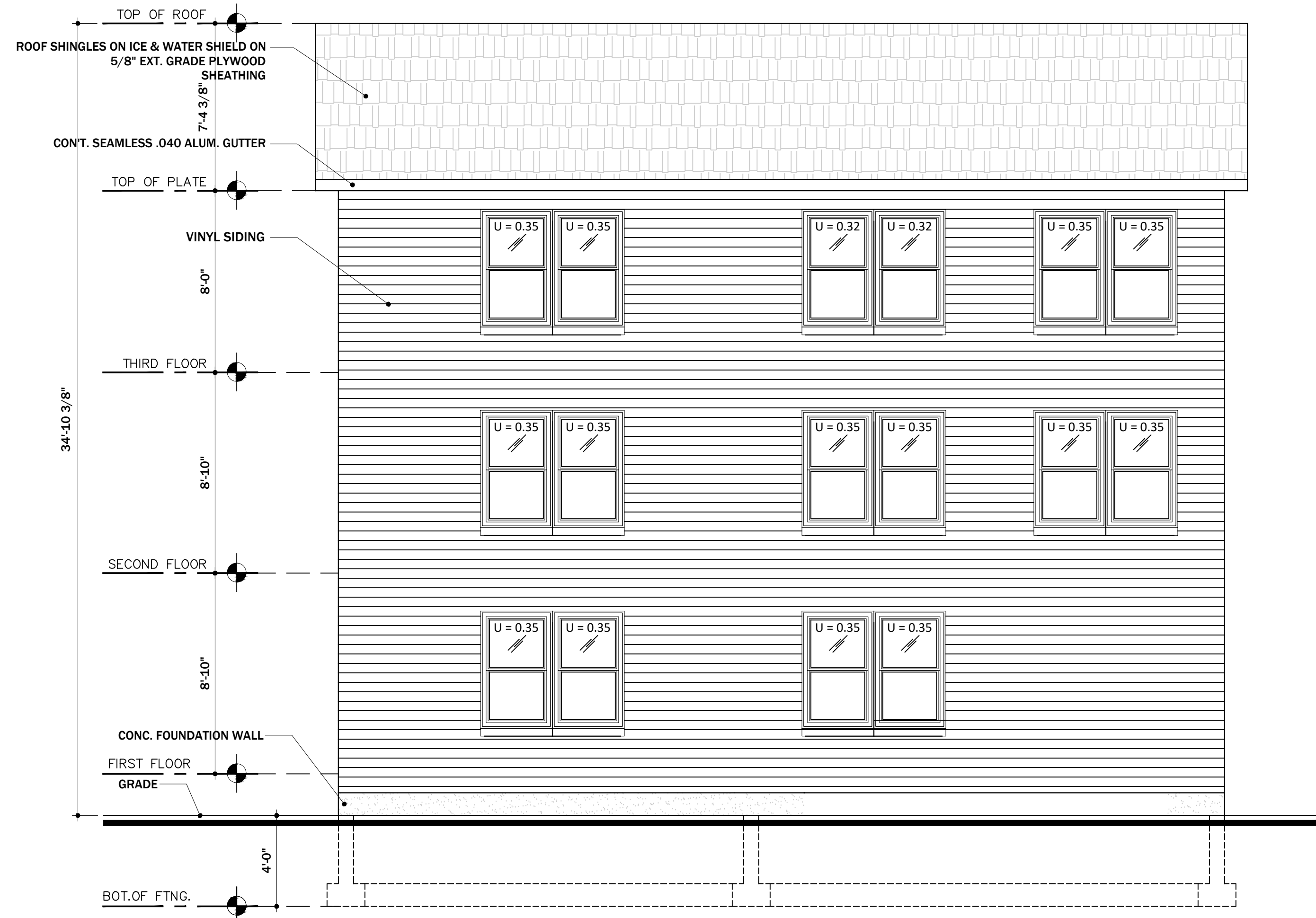
2 FRONT ELEVATION @ PARK AVE Scale: 1/4"=1'-0"
